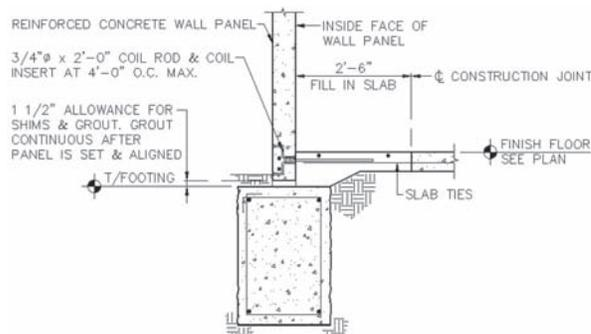
Typical panel to slab-on-grade connection.
